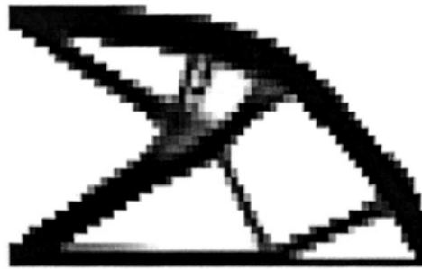
Fig. 16. The result by FTOP for the problem defined in Fig. 16 ( N_{\text{iter}} = 40 , N_f = 124 , L_{\text{opt}} = 3982.87 ).
